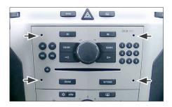
Put the radio release keys in the holes of OEM radio (see arrows)
