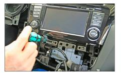
5. Remove all screws of OEM head unit
