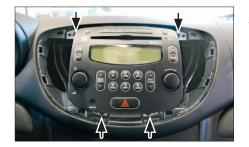
4. Remove the 4 screws (see arrows) fixing the OEM head unit
