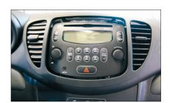
3. Remove the OEM center panel surrounding the OEM head unit
