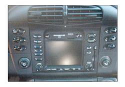
Insert Porsche radio release keys in the holes of the PCM head unit.
