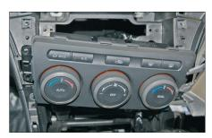
6. Remove the air condition control unit
