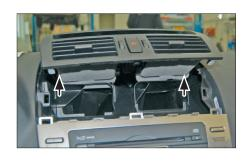
Remove the air vent unit above the OEM head unit
