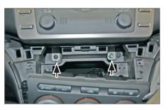
7. Remove the screws at the bottom of the OEM head unit.
