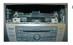
Remove the 2 screws at the top of the OEM head unit.
