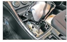
2. Remove the gear shift cover
