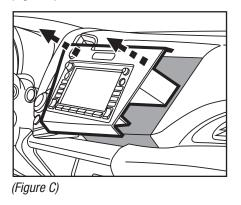
1. Remove the center top clip off of the factory radio and install onto the double din facia plate
