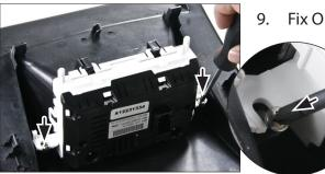
P. Fix OEM display with 2 screws
