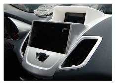
Connect all required circuit points of Double-DIN Navigation, mount it to Double DIN facia plate, place it on the dashboard.
