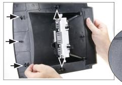
10. Remove clamps from Ford OEM panel. Place clamps on new facia plate
