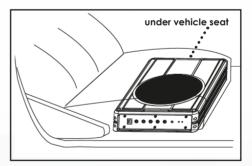
3. Mark the location for the mounting hole screws by positioning the cabinet where you wish to install it. Make a small mark to identify the position and remove the unit.
