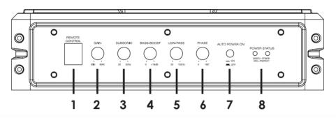
**1. REMOTE LEVEL CONTROL PORT -** Attach the included remote level control to adjust the volume level of the subwoofer independently.
