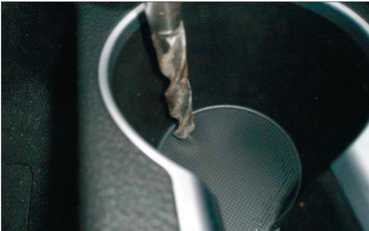
=> If the cup holder has a solid bottom you have to drill a hole (diameter of 18 mm) in order to install the USB connector cable
