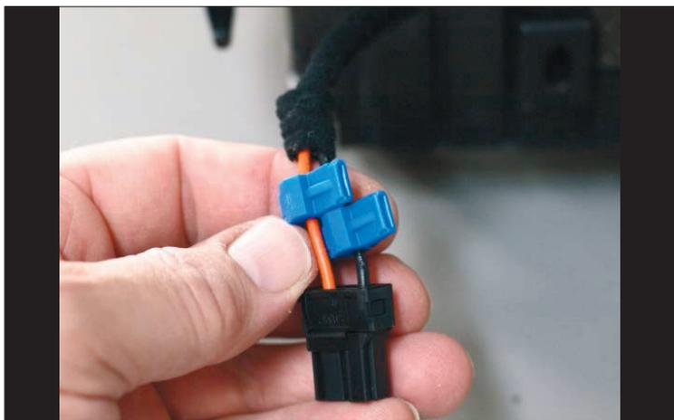
=> Disconnect the plug of the on-board socket and push down a bit the cable insulation
