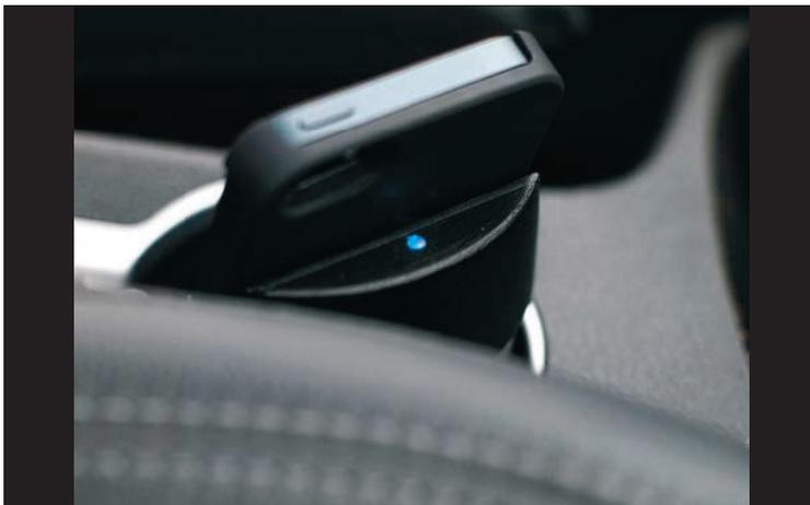
When Inserting a Qi compatible smartphone charging begins automatically and the LED turns from red to blue
