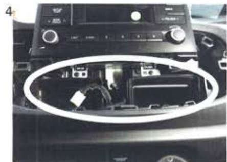
4 Remove and save the air-vents and the hazard lights button as shown in the picture.
