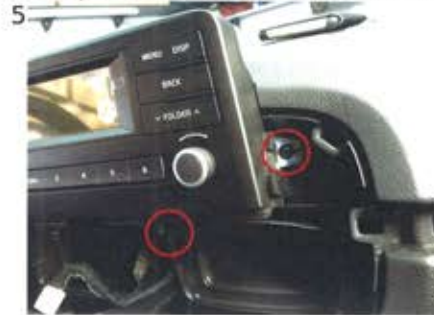
6 Take the supplied bracket and fix it on the supplied facia plate with the supplied screws. See the picture to check the position of the screws.
