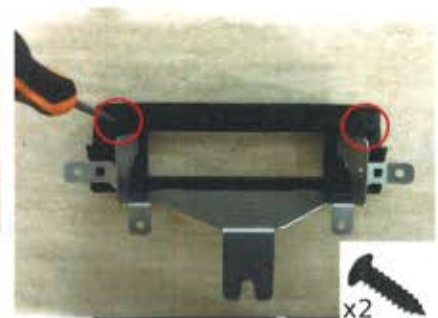
7 Take the bracket previously fixed and fix it on the aftermarket radio unit with the supplied screws (choose the appropriate type of screw between the two types supplied, see the picture below) on each side of the radio. See the picture to check the position of the screws.
