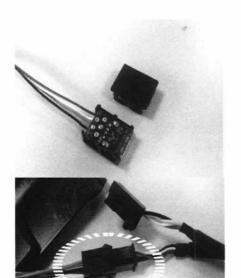
Take the PCB with USB plug and place it into the original housing .
