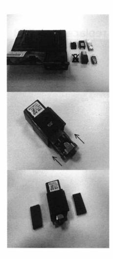
Take out the plastic panel of the Jack/USB interface and remove the two interfaces. Open the plastic covers as shown in the picture and take out the original PCBs. This removed plastic part marked with an X will no longer be required.
