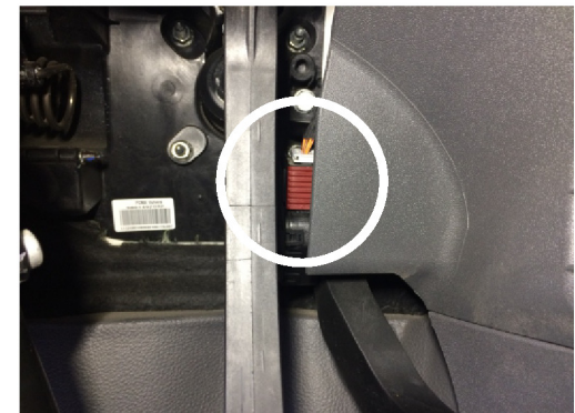
Dismount the original throttle connector from the pedal, and connect the enclosed Y cable. Mount the other end of the Y cable in the pedal.
