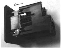
Take the rear plastic saved before and close it with the front plastic. You may need to exert some force to fit the black connector on the right position.
