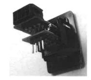
During this operation, adjust the distance between the two PCB, in order to facilitate the insertion of the part and fit the sockets to the holes.
