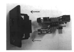
Take the new PCB and slide it into the original housing.
