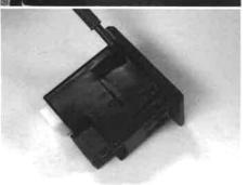
Take the original part and, in order to unhook the rear plastic, use a screwer by lightly lever into the slots as shown in the picture.
